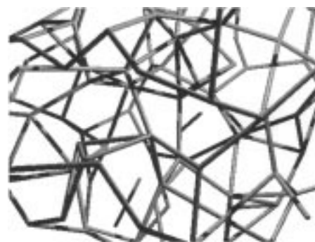
Figure 10. Statistical network of liquid water. Snapshot from molecular dynamics simulations.
