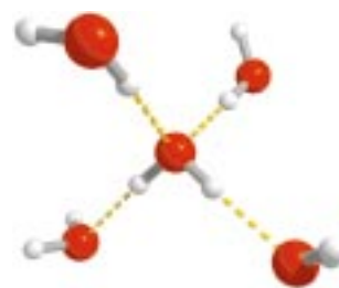
Figure 7. Tetrahedral configuration of water molecules spanned by two covalent bonds and two “lone pairs” of the central monomer.
