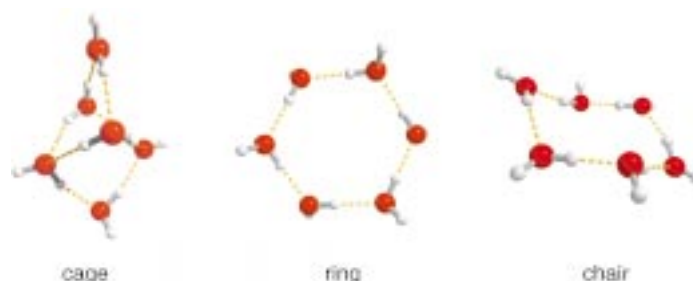
Figure 21. Experimentally found water hexamers: the cage structure detected in the gas phase, [146] the quasi-planar cyclic structure trapped in liquid helium, [147] and the chairlike cyclic structure measured in organic hosts. [148]
